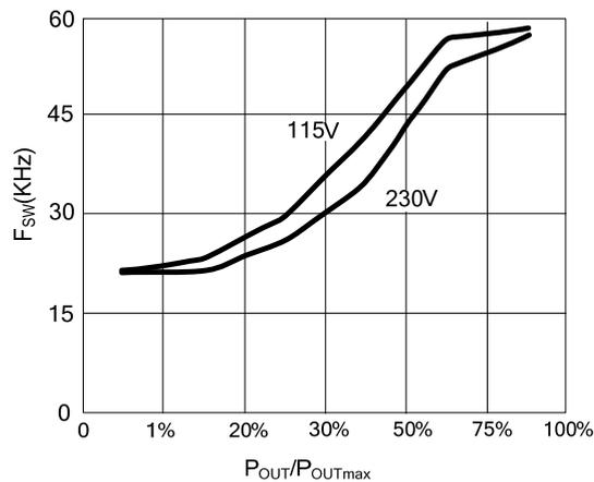
Fig.1 The relation curve between f<sub>SW</sub> and relative output power P<sub>OUT</sub>/ P<sub>OUT (MAX)</sub>
