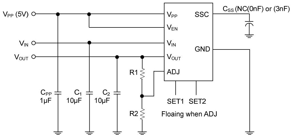
$$V_{OUT} = \frac{0.8(R_1+R_2)}{R_2} \text{ Volts}$$
